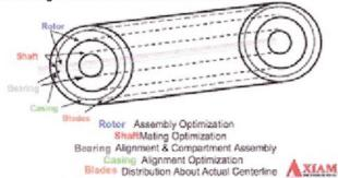
process variables, according to company material, consistently resulting in repeatable, straight and optimal builds on the first pass. Axiam's unique assembly processes build the engine core (all rotors, shaft mating, bearings/seals, casing, and optimized blade distribution) so that the turbine's dynamic and static structures are aligned about the actual centerline of rotation. As a result, the shop can better manage blade-tip gaps.
